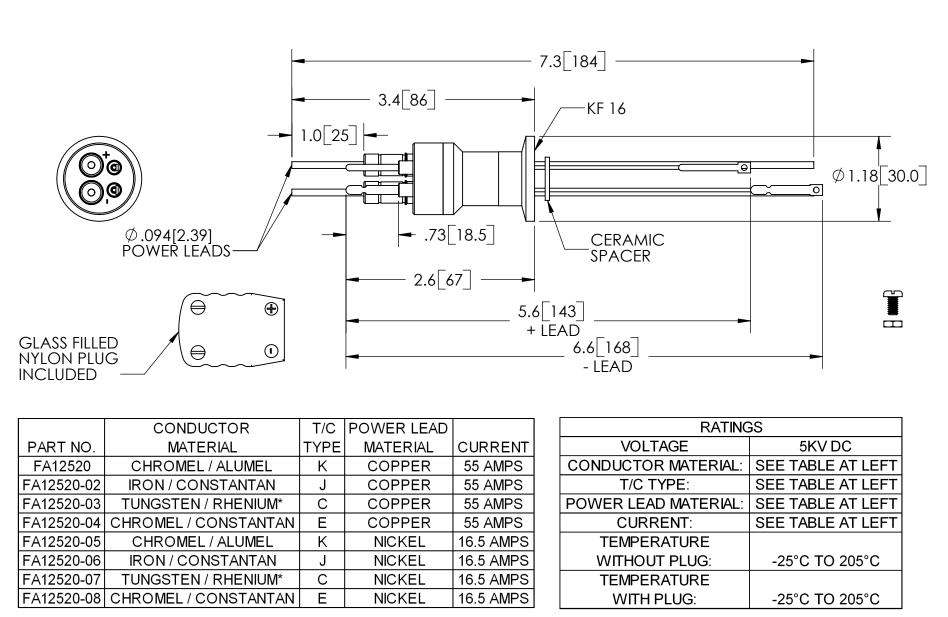
\*TYPE C USES COMPENSATING WIRE. MAXIMUM JUNCTION TEMPERATURE 250°C
